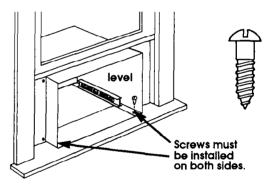
■ Lower window sash. Place level inside cabinet on the right side. There should be a tilt to the outside of approximately one bubble. Place the level on the left side and check.
